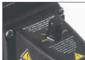
Close-up of variable-speed control found on the motors
