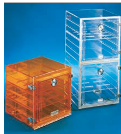
08900-52 Amber colored desiccators protect light-sensitive compounds from ultraviolet light.
